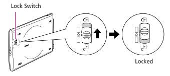
**WARNING** • Carrying or transporting the scanner without locking the scanning unit may damage it. Be particularly careful to lock the scanning unit when transporting the scanner in a vehicle.
